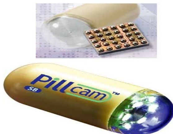
4. This semiconductor camera (a) crafted by Zarlink Semiconductor lies at the heart of Given Imaging's PillCam vitamin-sized capsule for gastrointestinal studies (b).
